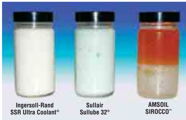
The first two oils are glycol-based and have difficulty separating from water, causing them to form damaging emulsions. SIROCCO™ quickly separates from water, increasing compressor protection.
