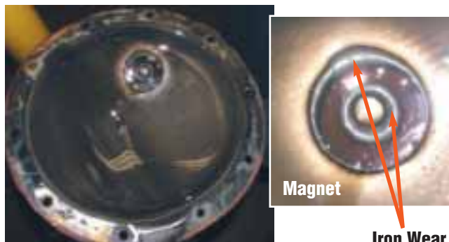
Differential gear lube sumps are equipped with magnets that attract metal wear particles.
