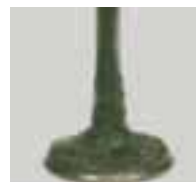
Intake valve before PI treatment.
