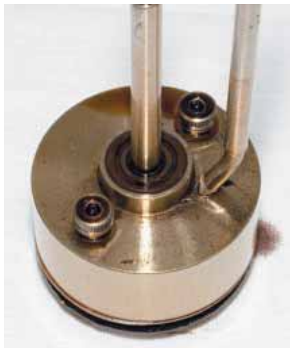
Texaco Havoline ATF left a covering of deposits following 1,012 hours of extended ABOT testing.
